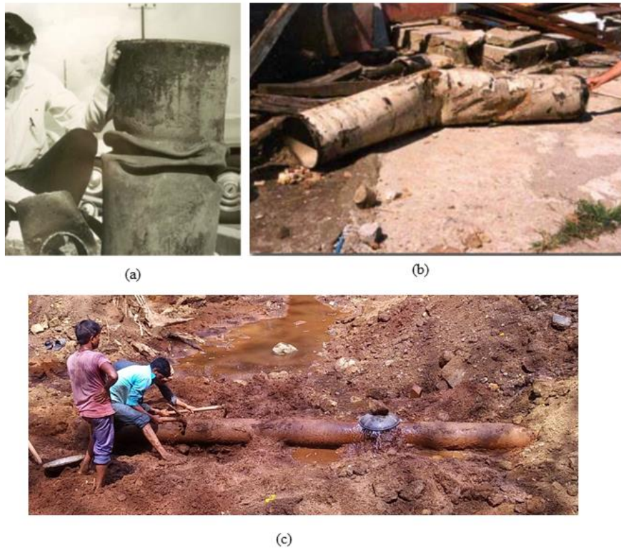
Fig. 1. (a) Buckling of steel pipe during 1971 Sanfernando earthquake (after Chenna et al. [31]) (b) Failure of pipe during 1999 Kocaeli Earthquake (after Chenna et al. [31]) and (c) Water leakage from pipe near IIT Bombay main building (3 June, 2019).
